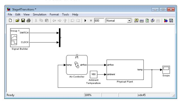
When you define one or more input events for a chart, Stateflow software adds a single trigger port to the block. External Simulink blocks can trigger the input events via a signal or vector of signals connected to the trigger port.
