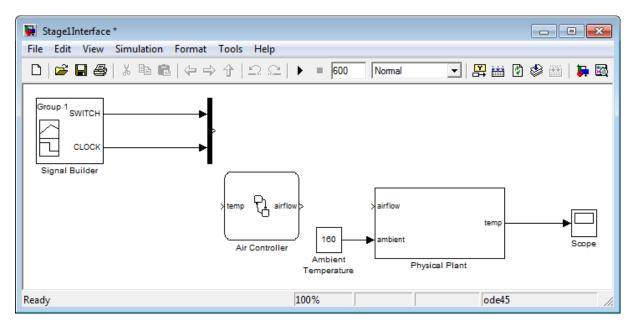
Notice that the input temp and output airflow have been added to the Stateflow block:
