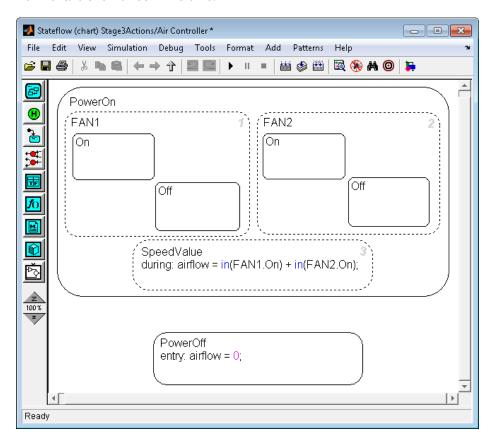
The Boolean expression in (FAN1.0n) is true — and its value equals 1 — if the On state of FAN1 is active. If FAN1 is not on — that is, its Off state is active or power is off — then in (FAN1.0n) equals 0. Similarly, the value of
