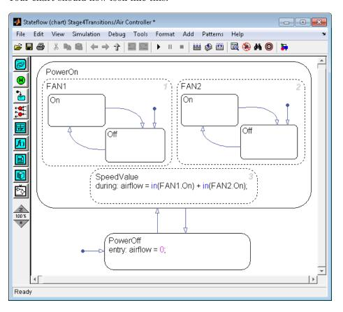
**Tip** The location of the tail of a default transition determines the state it activates. Therefore, make sure that your default transition fits completely inside the parent of the state that it activates. In the Air Controller chart pictured above, notice that the default transition for FAN1.0ff correctly resides inside the parent state, FAN1. Now consider this chart:
