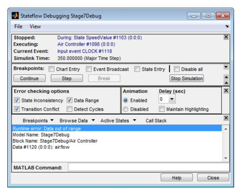
Simulation pauses after 350 seconds because of an out-of-range data error:
