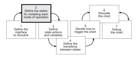
In phase 2 of this workflow, you define the states for modeling each mode of operation.
