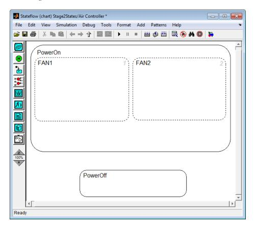
**Note** Your chart might not show the same execution order for parallel substates FAN1 and FAN2. The reason is that, by default, Stateflow software orders parallel states based on order of creation. If you add FAN2 before FAN1 in your chart, FAN2 moves to the top of the order. You will fine-tune order of activation in a later exercise, "Setting Explicit Ordering of Parallel States" on page 4-17.
