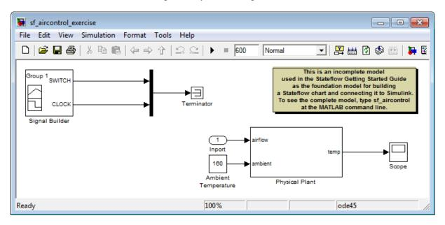
The model is incomplete because it does not include the Stateflow chart that you will build as you work through the exercises in this guide. Instead, the model contains several nonfunctional blocks: the Terminator, Inport, and Annotation blocks.
