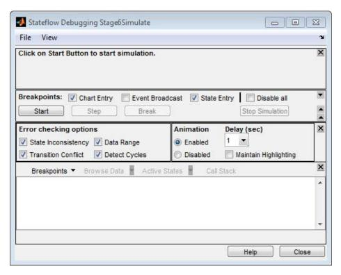
The **Browse Data** option appears grayed out, but becomes active when simulation pauses at a breakpoint. You will use this option in "Simulating the Air Controller Chart" on page 8-9.
