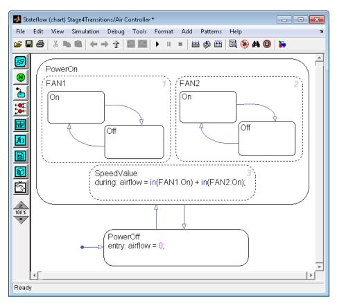
5 Repeat the same procedure to add default transitions at the top edges of FAN1.0ff and FAN2.0ff.
