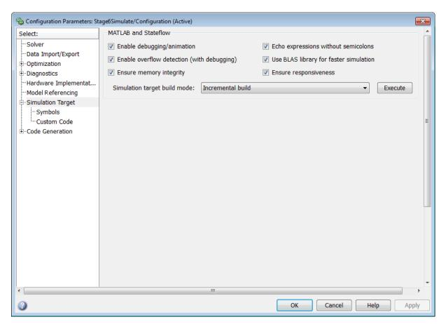
**Note** This dialog box is used to configure Stateflow software for building targets. A target is a program that executes a Stateflow chart or a Simulink model that contains a Stateflow chart. Stateflow software builds a simulation target that you use to simulate your Stateflow application. For more information, see "Building Targets" in the Stateflow User's Guide.
